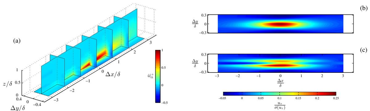
Figure 2: (a) Iso-contours of  $u^+$  velocity fluctuations conditionally averaged on a high skin-friction event. Two dimensional high skin-friction footprint at the wall, (b) unmodified flow; (c) modified by the ‘jet’
