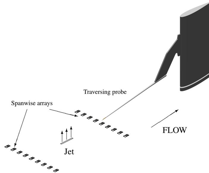
Figure 1: Schematic drawing of the experimental setup (figure not to scale)
